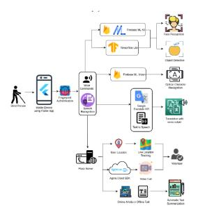
This is a cross platform mobile application which makes use of device's camera to perform various operations that help in day to day activities for the visually impaired. The idea is not just restricted to a simple mobile application as a system can be integrated with various other devices that can work on a live image capturing pictures manually cars) technique rather than taking pictures manually again and again.
